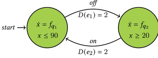
Figure 2: The dHA for the heating system
