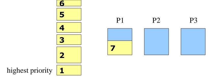
■ Select the processor on which the assigned utilization is the lowest
