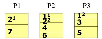
■ Select the processor on which the assigned utilization is the lowest
