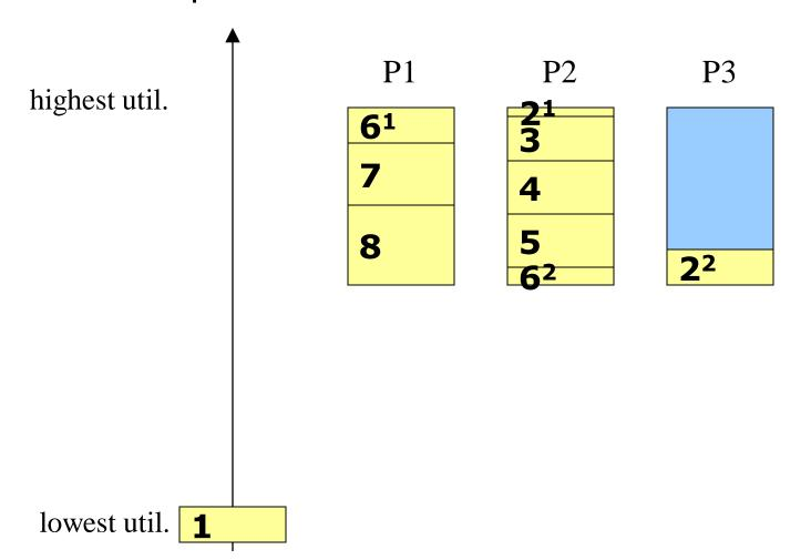
Pick up one processor, and assign as many tasks as possible
