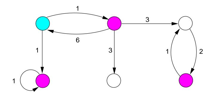
determine the bottom strongly-connected components
