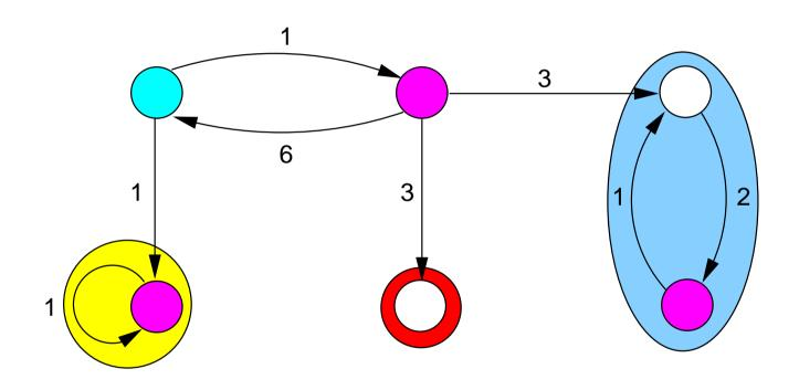
$$s \models \mathbb{L}_{>\frac{3}{4}}(\textit{magenta}) \quad \textit{iff} \quad \underbrace{\Pr\{s \models \Diamond at_{yellow}\}}_{\frac{2}{3}} + \frac{2}{3}\underbrace{\Pr\{s \models \Diamond at_{blue}\}}_{\frac{1}{6}} > \frac{3}{4}$$
