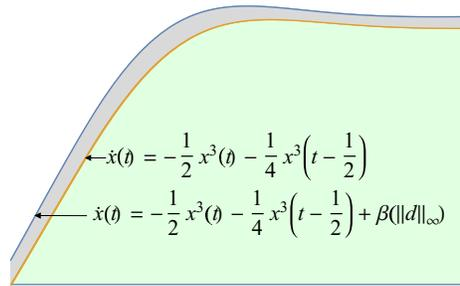
**Figure 1** An example of the safe set  $\mathcal{C}$  and the corresponding input-to-state safe set  $\mathcal{C}_d$ . The green region is set  $\mathcal{C}$ , Green + Grey region is set  $\mathcal{C}_d$ .
