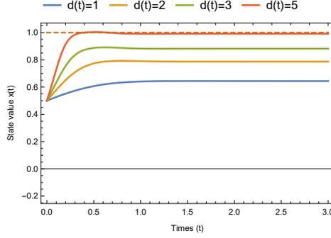
**Figure 3** State evolution of the system for different disturbances when applying the ISSf controllers. The dashed lines correspond to  $x = -1$  and  $x = 1$ , the boundaries of the safe set.
