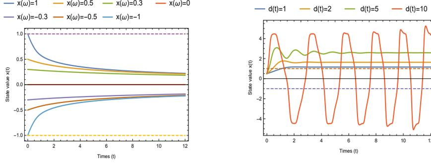
**Figure 2 Left:** state evolution of the system for different initial conditions  $x(\omega)$ . The dashed lines correspond to  $x = -1$  and  $x = 1$ , the boundaries of the safe set.
