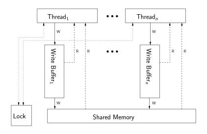
The write buffer explains how "reads can pass over writes".
