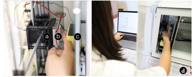
Figure 1: Experimental device (a: 40mm*40mm FSR sensor, b: 40mm*40mm TEC plate with a water-cooling equipment, c: printer plate with a finger holder) and (d) study setup (user separated from the experimental device by a board)
